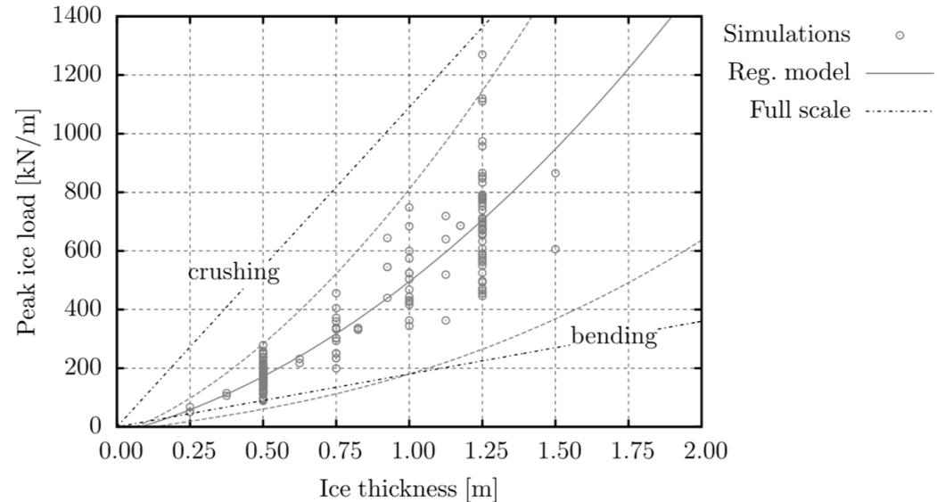
Left: DEM with Lab data from Aalto Ice Tank (Saarinen, 2000)
